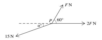
Three coplanar forces of magnitudes F N, 2F N and 15 N act at a point P, as shown in the diagram. Given that the forces are in equilibrium, find the values of F and  $\alpha$ . [6]
